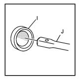
Insert the open end of the extension (J) through the hole in the rear bumper (I) (hoist shaft access hole).
